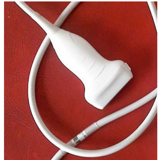
Figure 1: A linear ultrasound probe.
